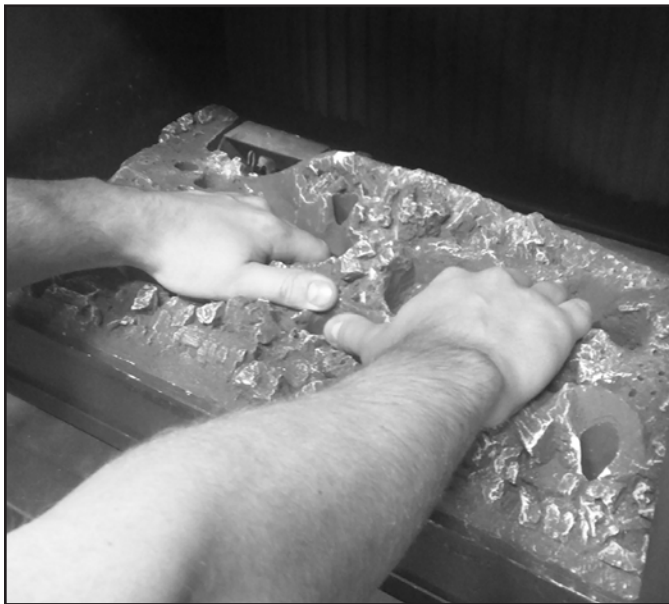
Figure 25. Burner Removal - Correct Hand Placement
