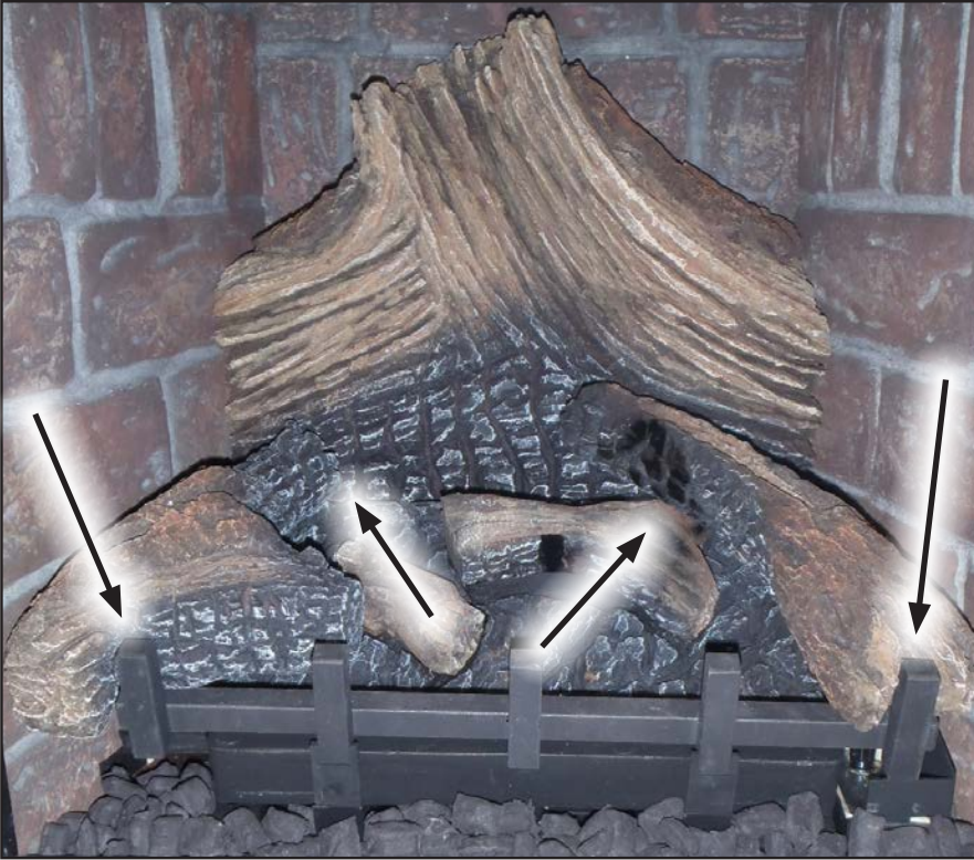
Figure 44. Third Stage Log Set Installation.
