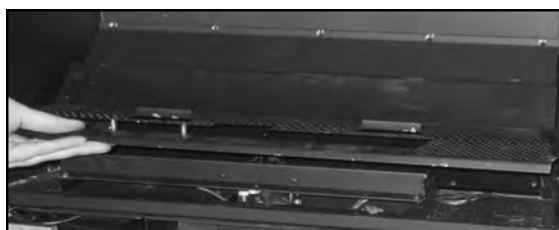
Figure 56: Burner Tray Installation.
