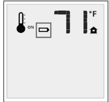
Figure 17: Low Battery Indicator.
