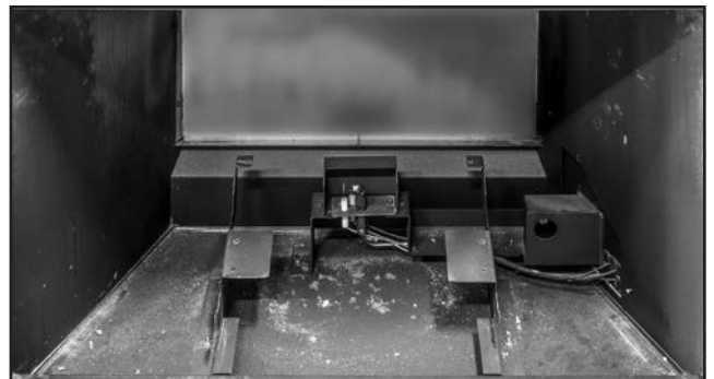
Figure 56: The rear liner can now be removed. Use a vacuum to clean up the bare firebox if needed.
