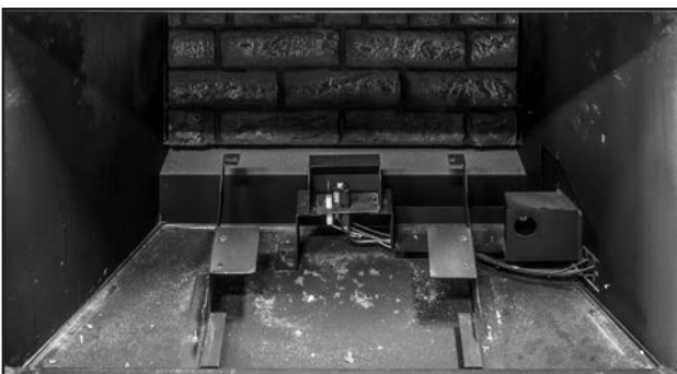
Figure 55: Lift the burner off the mounts and pull it out of the inlet box. The unscrew the panel brackets (T20's) from each side of the baffle to remove the left and right side liners.
