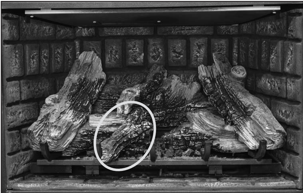
Figure 64: Rest the center top log on top of the left mid log making sure to align the bottom with grate arm.
