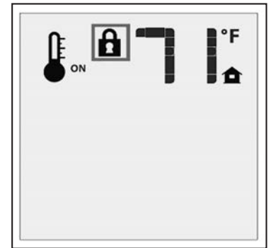
Figure 16: Remote Control Locked.
