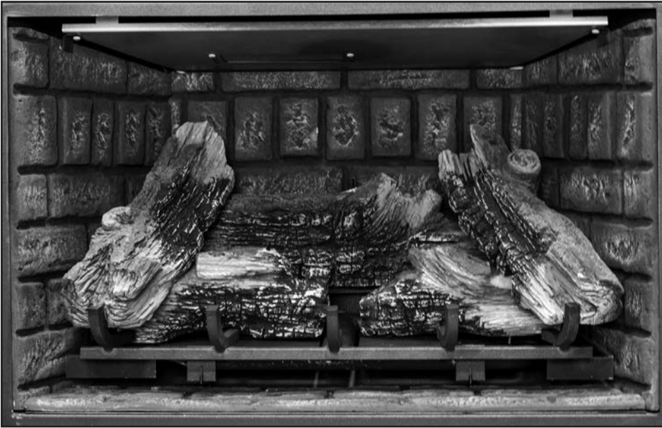
Figure 57: Install the right top log on top of rear log and right mid log. Locate the bottom on the far right grate arm.
