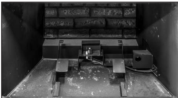
Figure 52: Lift the burner off the mounts and pull it out of the inlet box. The unscrew the panel brackets (T20's) from each side of the baffle to remove the left and right side liners.
