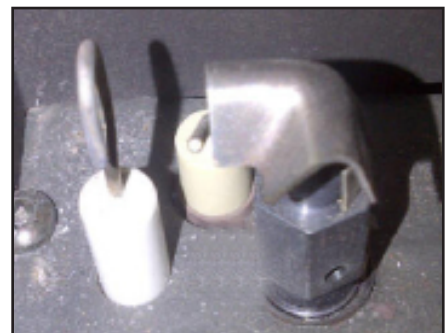
Figure 23: Proper Pilot Position
