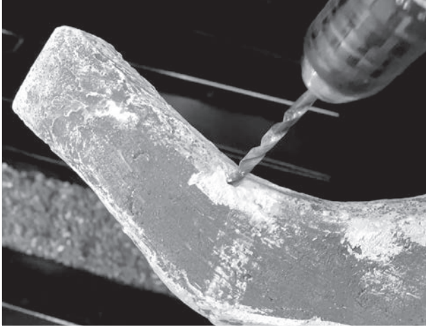
Figure 76: Using a 5/16 drill bit, drill a hole 1in deep in the Rear Right Log as shown above.
