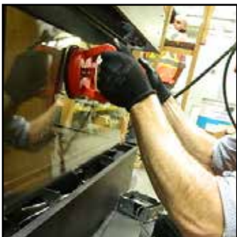
Handle glass with supplied vacuum clamps
