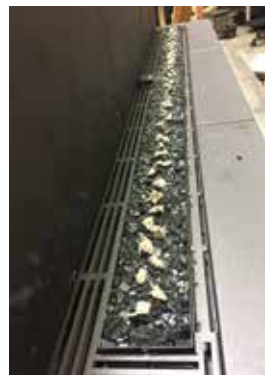
Burner covered with Fireglass and glowing wool
