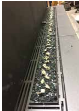
Burner covered with Fireglass and glowing wool
