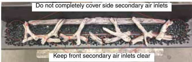
Correct Black Coal placement
