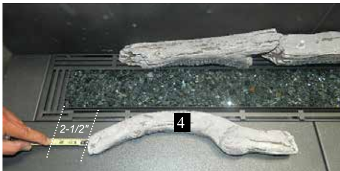
Log 4 to edge of burner
