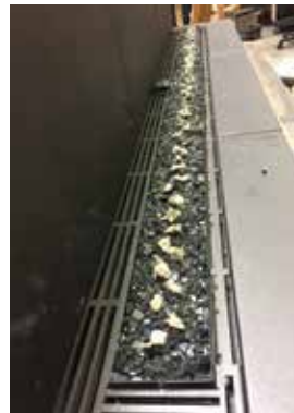
Burner covered with Fireglass and glowing wool
