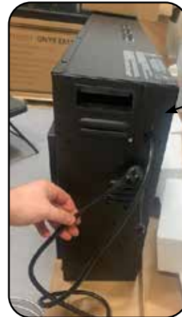
Wire Harness & Cover Plate Reinstalled.
