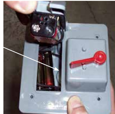
Slide 1st battery pack to the right.
