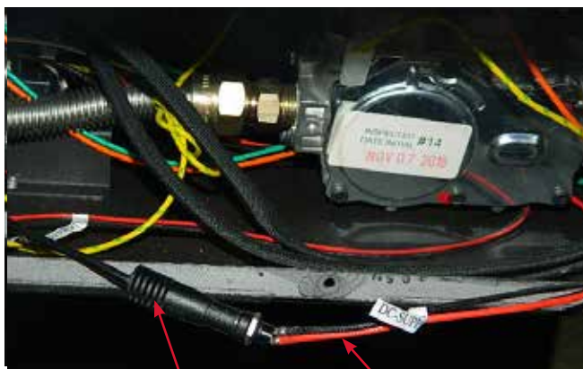
DC supply wire from wiring harness
